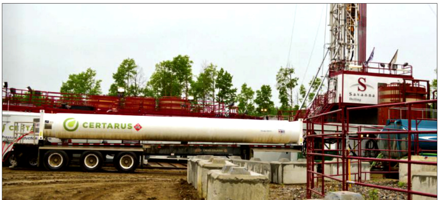
This Certarus trailer carrying compressed natural gas (CNG) powers a drill rig north of Rocky in June. CNG offers drilling rigs an alternative fuel to diesel. Rigs need to be outfitted with a bi-fuel system to accommodate the natural gas, but once it is installed the system saves money and reduces emissions.
